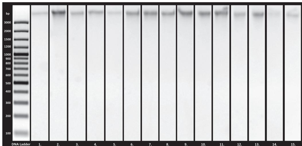
**Figure 4.** Visualisation of isolated yeast DNA (*Saccharomyces cerevisiae*) using the S.M. Aljanabi and I. Martinez universal protocol in 1.8% Agarose gel by horizontal electrophoresis. DNA size marker/Ladder: Gene Ruler 100bp. Plus DNA Ladder (Thermo Scientific).
